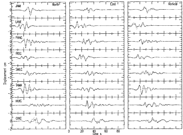
Figure 3. Strong-motion seismograms (solid lines) and synthetic seismograms (dotted lines). Synthetics and observations are plotted on the same scale. The synthetics correspond to the solution shown in Figure 2.
